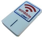
Useful for mobile application (outreaches). Has a built in battery for 4-5 hours. It comes with a 240V charge adaptor. Range: 30m open field.
