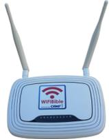
Useful to make the WIFIBible available to a bigger area as it has a range up to 200m open field. It comes with a 240V power adaptor and works a little bit faster than its little brother.
